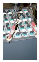
Typically steel trays (crates) are used in railway vehicles. Battery trays made of plastic are also used in railway applications and available at BAE. Especially in Germany plastic trays are quite common.
